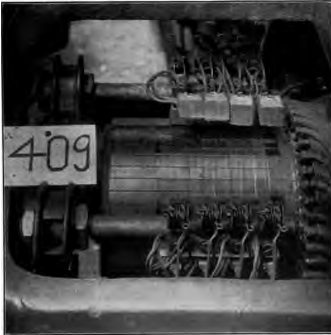
FIG. 93.—Scored commutator surface resulting from exposure of the machine to a blast of concrete dust. Note also the scoring on the brush faces.
